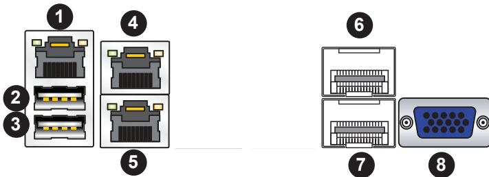
Figure 5-2. Rear Panel I/O Ports
