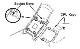
Once they are aligned, carefully lower the CPU straight down into the socket.
