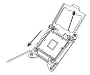
Using your thumb and index finger, hold the CPU by its edges. Align the CPU keys, which are semicircle notches, against the socket keys.
