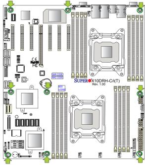
**Caution:** 1) To avoid damaging the motherboard and its components, do not use a force greater than 8 lb/inch on each mounting screw during motherboard installation. 2) Some components are very close to the mounting holes. Please use caution to prevent damage to these components when installing the motherboard to the chassis.
