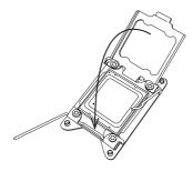
Push down and lock the lever labeled "Close 1st"
