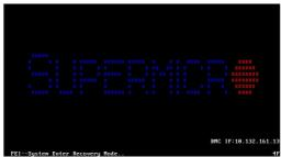
**Note:** On the other hand, if the following screen displays, please load the "Super.ROM" file to the root folder and connect this folder to the system. (You can do so by inserting a USB device that contains the new "Super. ROM" image to your machine for BIOS recovery.)
