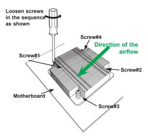
Notes: 1.) For optimized airflow, please follow your chassis airflow direction to properly install the heatsink. 2.) Graphics shown in this manual are for reference only. They may or may not look the same as the components installed in your system.
