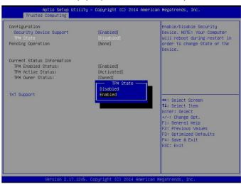
You must save your changes and reset for the changes to take effect. Scroll to the Save & Exit tab and select "Save Changes and Reset." The TPM is now enabled.
