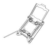
Warning: You can only install the CPU inside the socket in one direction. Make sure that it is properly inserted into the CPU socket before closing the load plate. If it doesn't close properly, do not force it as this may damage your CPU. Instead, open the load plate again to make sure that the CPU is aligned properly.
